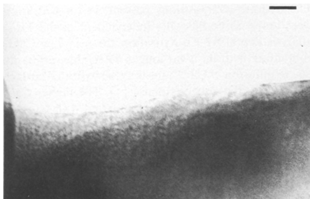
Figure 6 Micrograph of surface layers ( \text{CaO}/\text{SiO}_2 = 0.8 ) at 5 h; bar = 10 nm.
